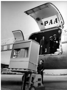
It held 50 24-inch hard disks that spun and 1200 RPM (today's drives spin at 5400 to 15,000 RPM). Its total storage capacity was a whopping 3.75 megabytes. Not to be confused with today's gigabyte-sized hard drives.
